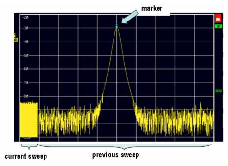
If the test software reads the trace data under such conditions, the resulting array of values consists of a mixture from two subsequent measurements. The data is obviously invalid.
