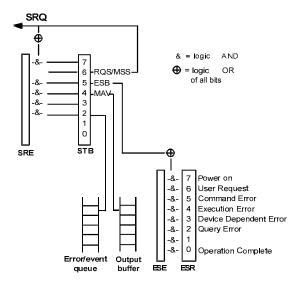
Bits of the Status Byte (STB) are masked with the contents of the Service Request Enable (SRE) register and combined with a logical OR operation into the RQS/MSS (Master Status Summary) bit. If this bit is set, the instrument issues a service request.
